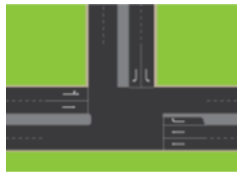
Figure 1: A typical three-legged intersection with a right-turn-bay
