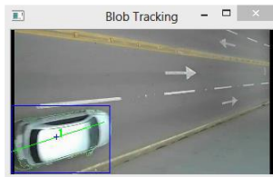
Figure 4: The vehicle detection with the bounding box
