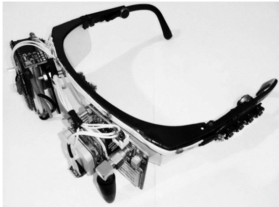
Figure 7: Prototype wearable device developed to validate the haptic navigation algorithm
