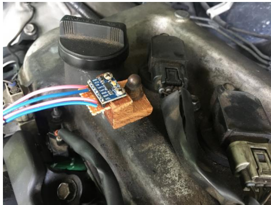
Fig 2: Accelerometer fixed rigidly to the engine block.
