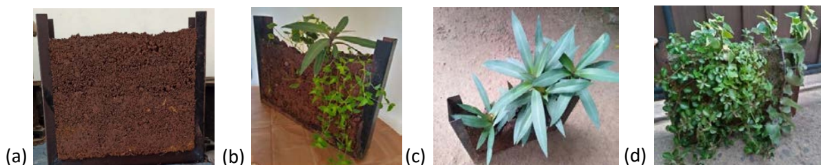
Fig 1: Prepared Slip Form Wall Panels. (a) before cultivation, (b, c, d) after cultivation
