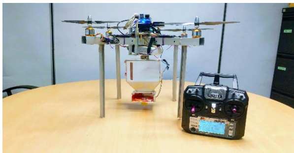
Fig. 1. Completed drone attached with the Raspberry Pi, seed dispenser and the transmitter.
