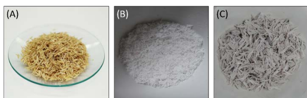
Fig. 1. Images of (A) acid-washed and dried RH, and RHA (i.e. sintered RH) (B) with and (C) without acid washing
