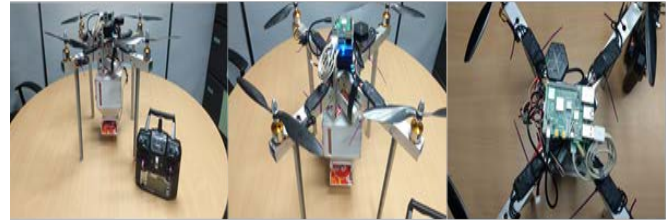
Fig.3. Completed drone attached with the Raspberry Pi and the transmitter
