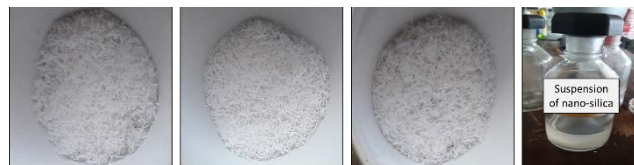
Fig. 2. Images of RHA washed using (A) fresh, (B) twice, and (C) thrice used acid, and (D) the milky suspension of ensuing nano-silica
